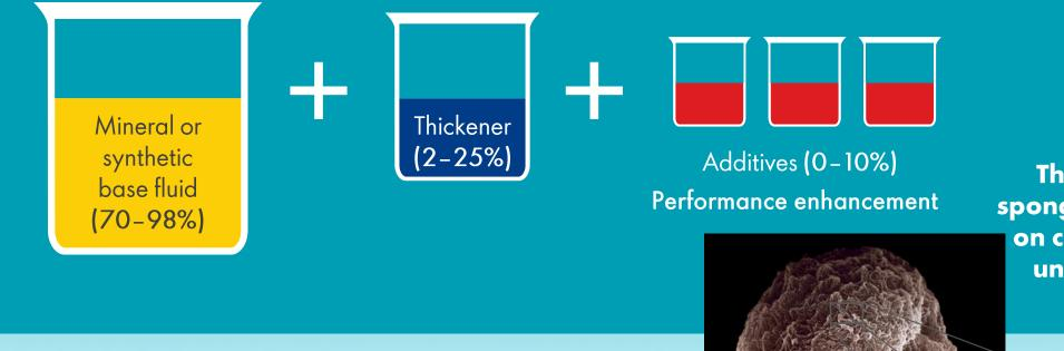
The thickener acts like a sponge, holding the base fluid on components, releasing it under pressure and then absorbing it.
