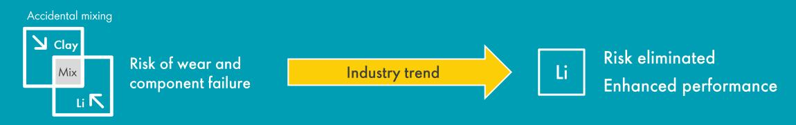
Aircraft manufacturers recommend that greases with different thickeners are **not** intermixed.
