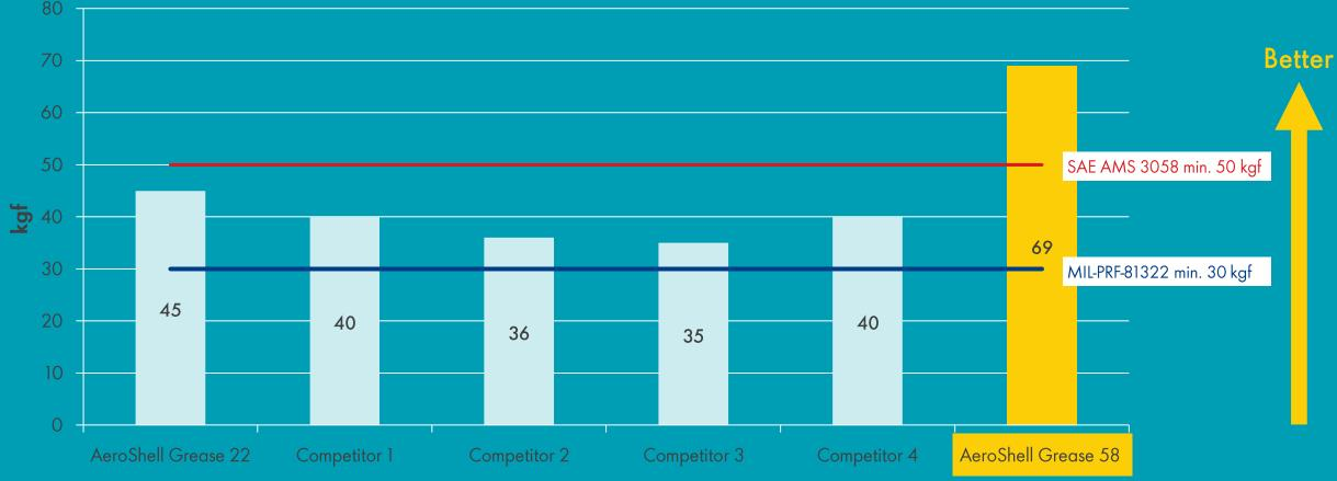
AeroShell Grease 58 supports higher loads compared with MIL-PRF-81322 approved greases.
