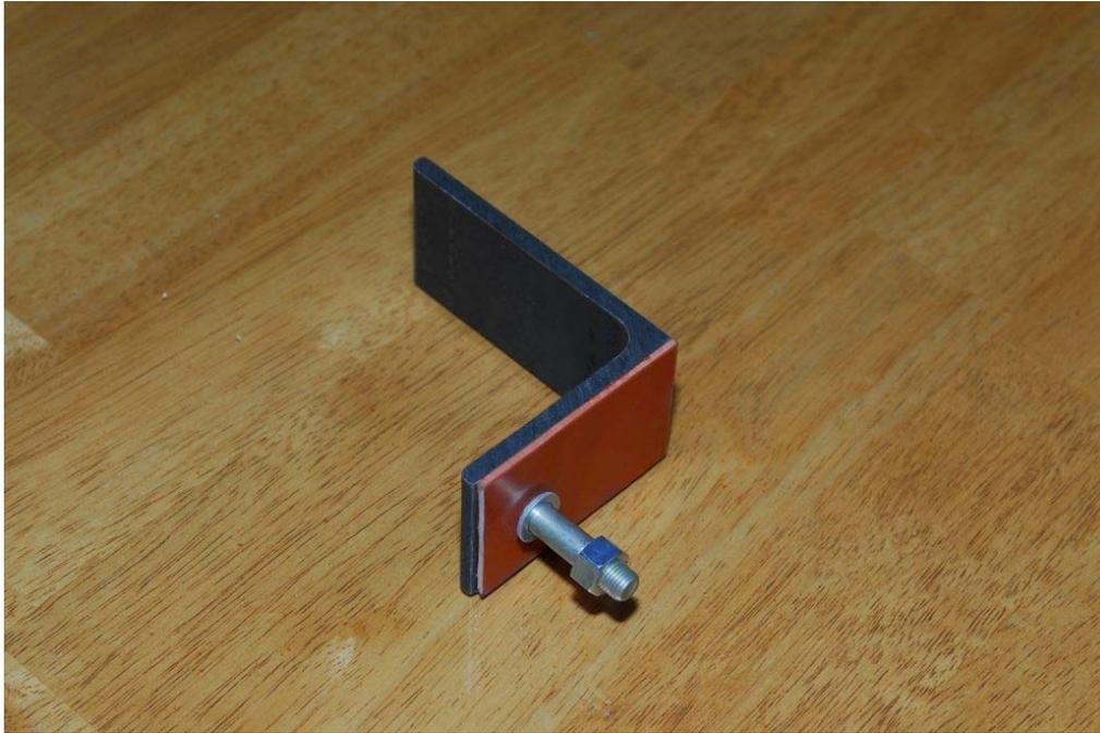
Figure 1. Nose Gear Jack Adaptor
