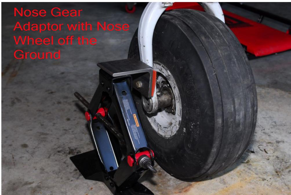
Figure 2. Nose Gear Adaptor In Use
