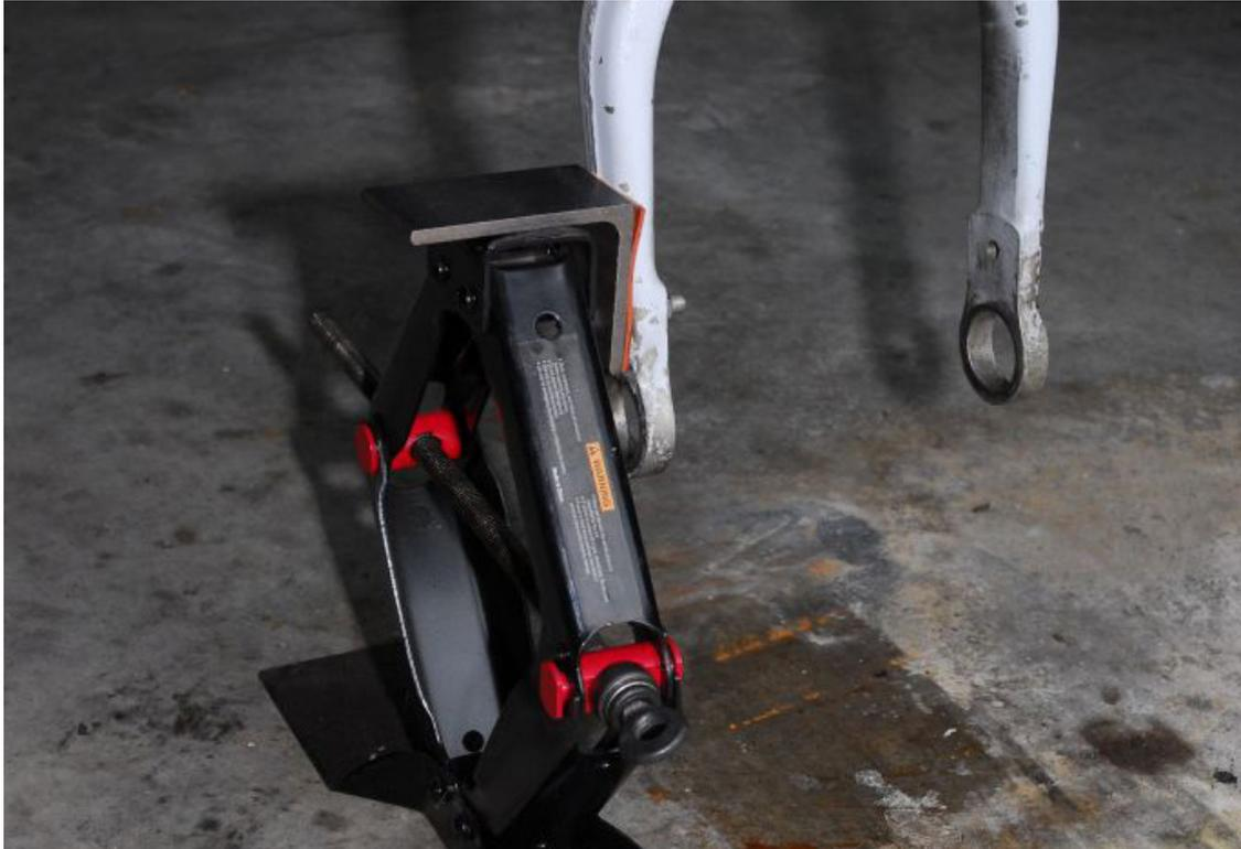
Figure 3. Nose Gear Adaptor With Wheel Removed
