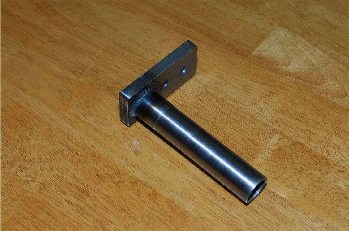
Figure 5. Main Gear Axle Tube Jack Adaptor
