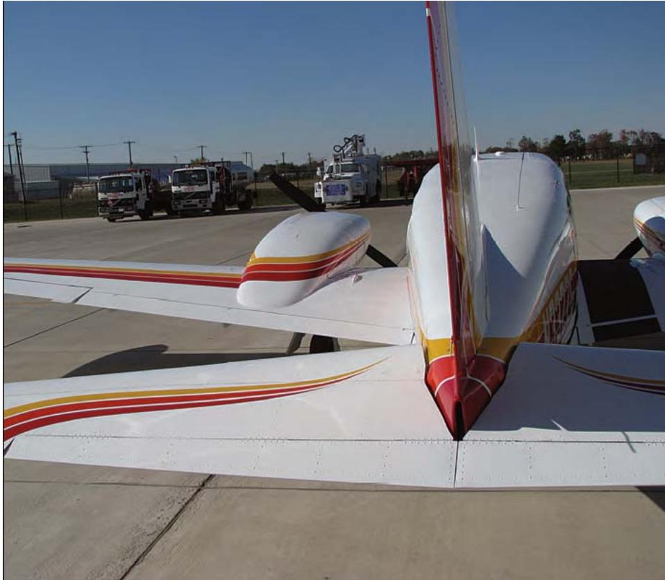
*This after-shot shows how the inboard cowl and stab design flow well.*
