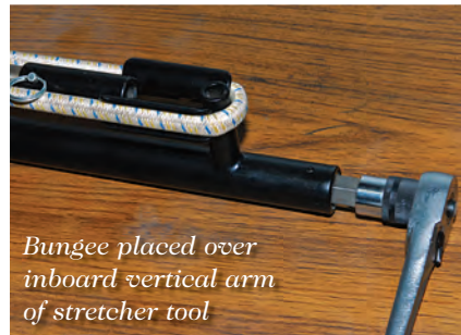
Installer tool in place on stretcher tool
