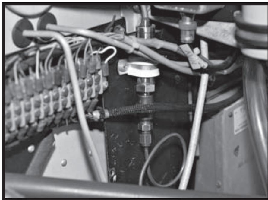
*Figure 5: Fuel pressure transducer on nose compartment firewall.*
