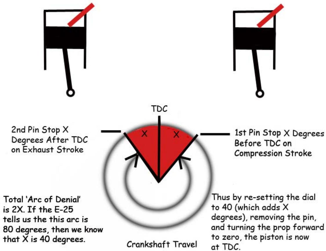
Figure 2 Timing Diagram
