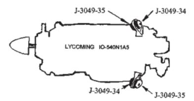
Note: There are differences in stiffness in the rubber compounds used in the sandwich mountings, so it is important to place the J-3049-35 sandwich mountings only in the top forward and bottom aft locations, and the J-3049-34 sandwich mountings only in the bottom forward and top aft locations.
