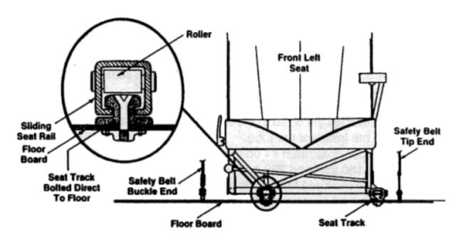
Extract from Piper Drawing #26652 Seat Installation
