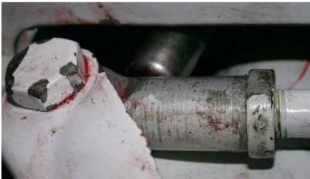
The main landing gear side brace link assembly rod end. If lubed correctly, it should move freely.
