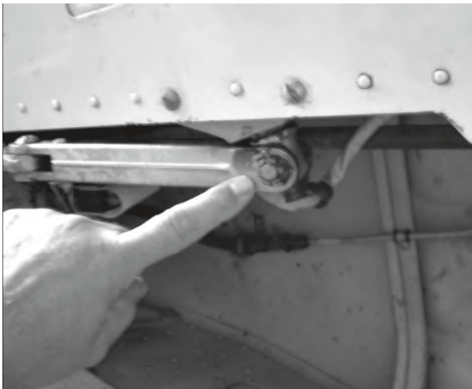
The clevis screw at the side brace stud
