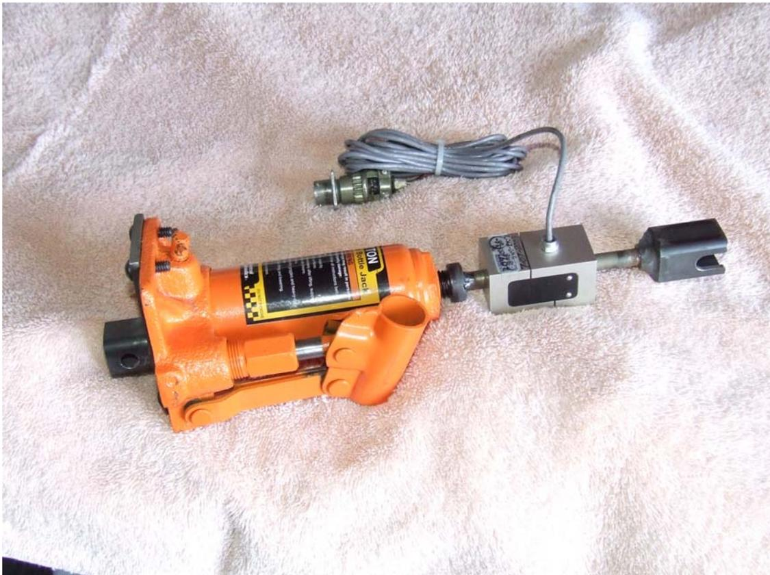
*Figure 2 Gear Retraction Test Setup using Hydraulic Jack and Load Cell*
