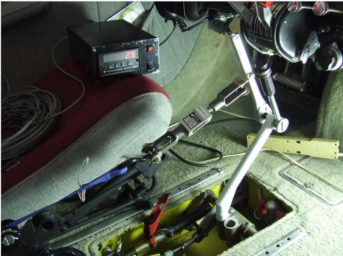
*Figure 1 Gear Retraction Test using Load Cell and Ratcheting Strap*
