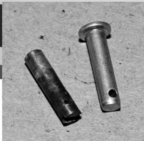
Figure 5a: Hinge pin and clevis pin compared (left).
