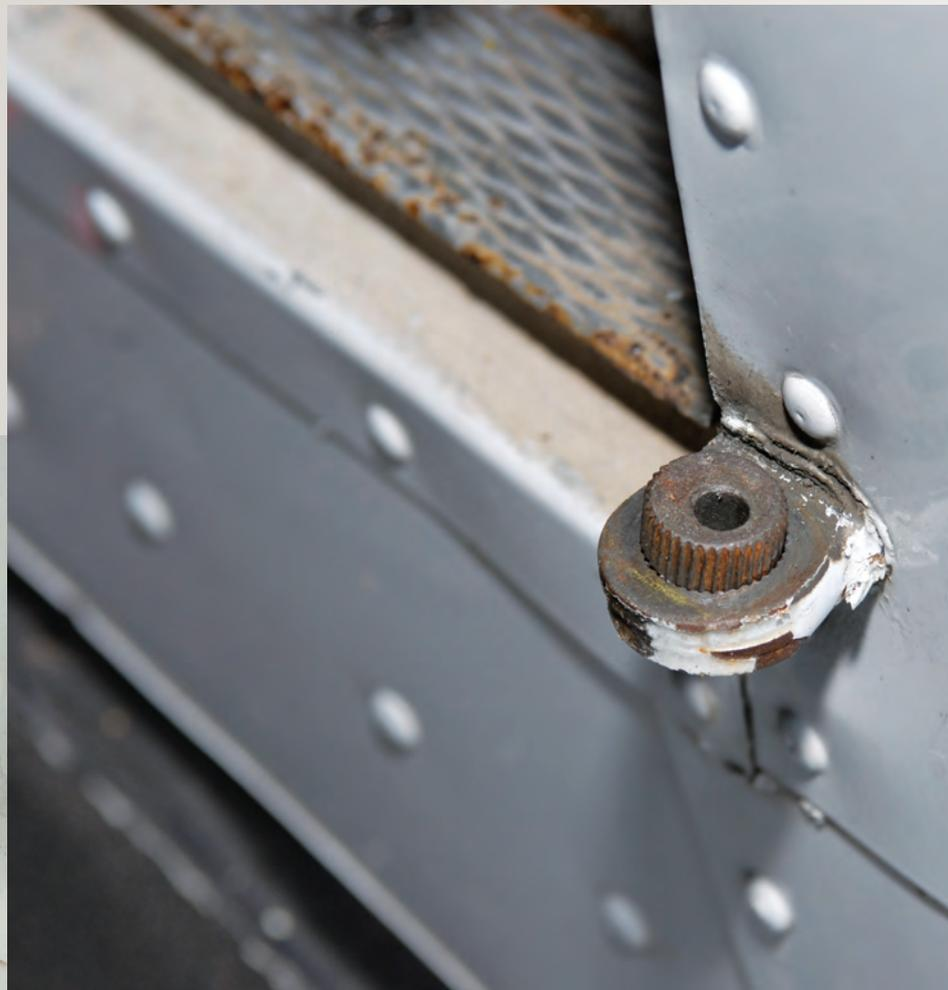
*Figure 1: Eccentric bushing pushed out of hinge tongue. Note the serrated edges and the eccentric location of the opening (above).*
