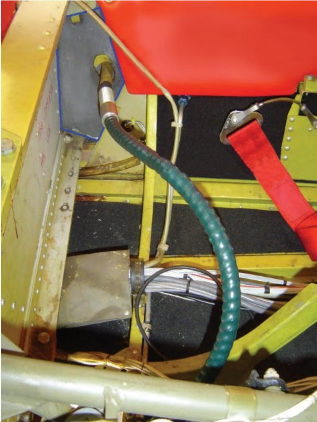
*FIGURE 3: This is the cover (blue outline) that should be found at this location. See discussion. Landing gear conduit (right side) shown at fuselage entry/exit point*
