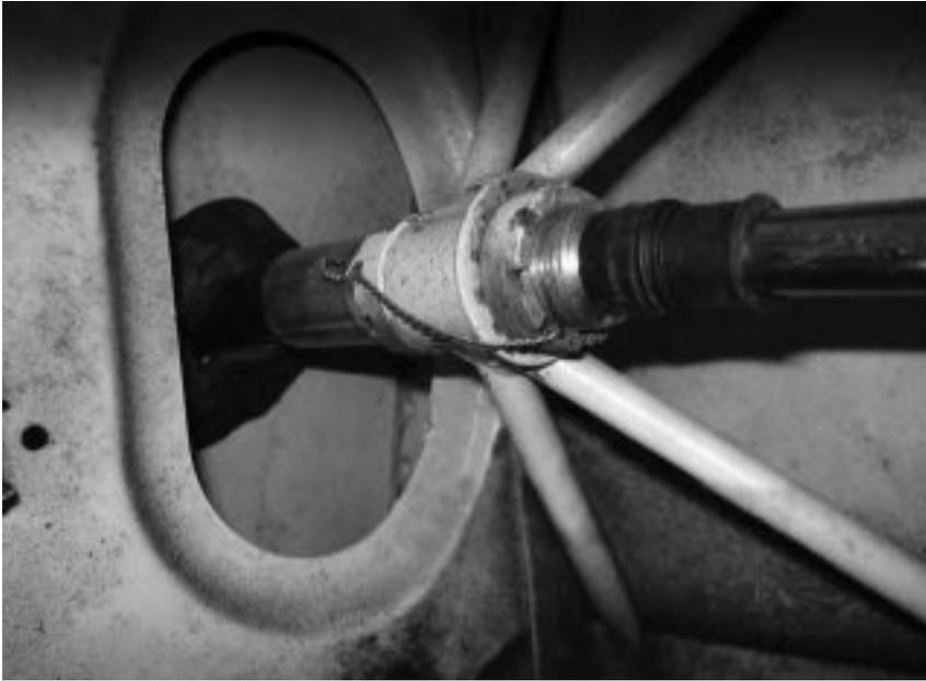
*FIGURE 4: Use "duct seal" here which will also reduce cabin draft somewhat and possibly keep wildlife from nesting inside the fuselage.*
