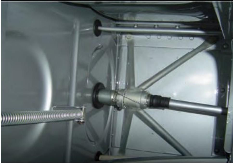
*FIGURE 2: Also make covers for the kidney-shaped opening in the root rib. These covers will benefit cabin-draft reduction.*
